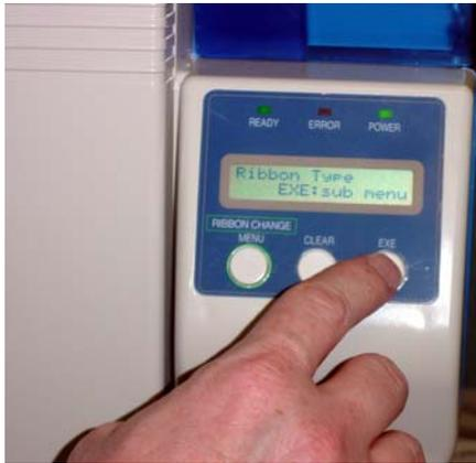
5. Press the Menu button until “H. Roller1 Ribbon” is displayed. The laminate ribbon type may be selected by pressing the EXE button. The available types are:
